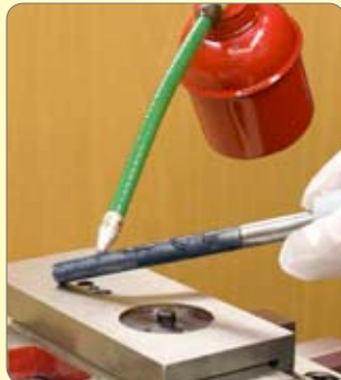
153. Fit adjusting screws and adjust so slide can be moved back and forth easily by hand.
