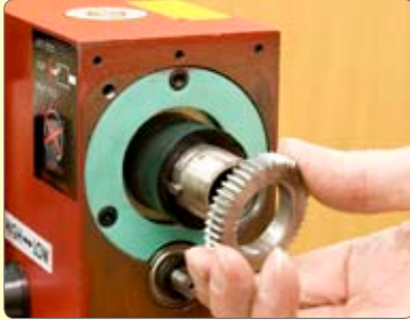
46. Remove Spindle Gear.
