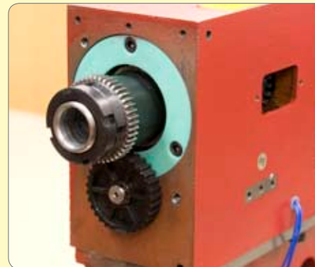
72. Fit plastic drive pulley, secure with circlip.
