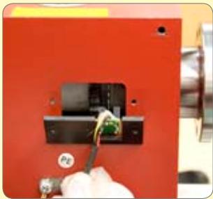
79. Check the speed encoder disk aligns with the pick-up and fit.
