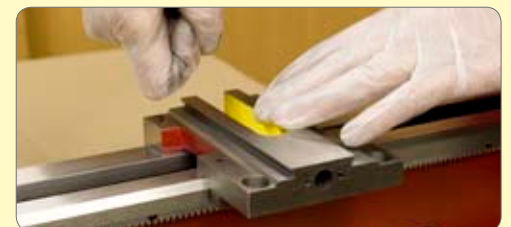
89. Place the saddle on the bed and check to see how it sits.
