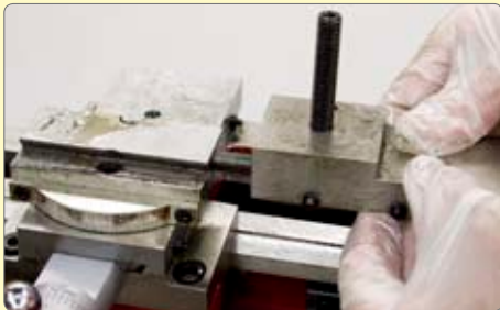
10. Remove compound slide and gib strip.
