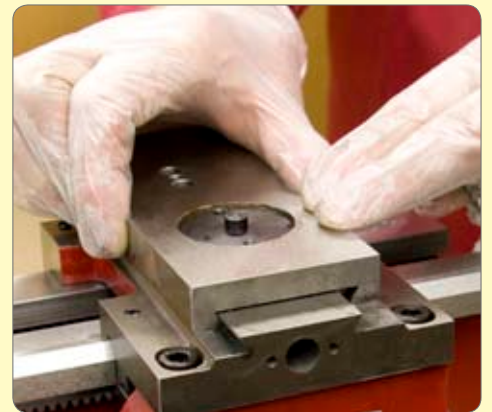
153. Fit adjusting screws and adjust so slide can be moved back and forth easily by hand.
