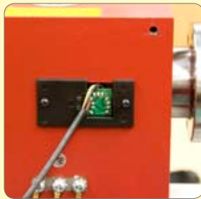
79. Check the speed encoder disk aligns with the pick-up and fit.
