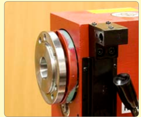
49. Using a hole in the spindle flange for access to the 3 fixing screws, remove the front bearing cover.
