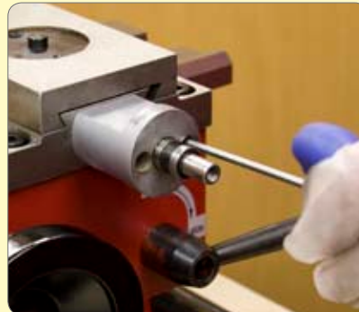
155. Assemble onto the saddle.
