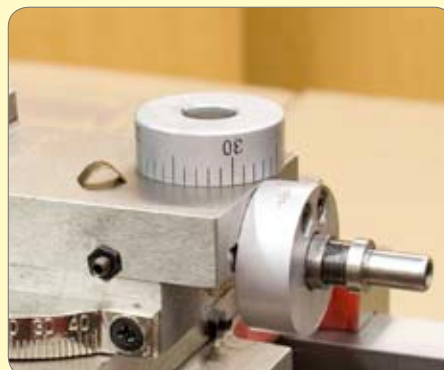
173. Assemble and fit the micrometer dial and friction clip to feed screw.
