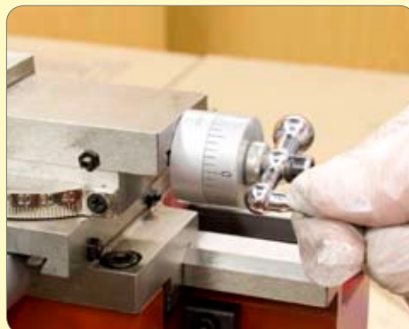
173. Assemble and fit the micrometer dial and friction clip to feed screw.
