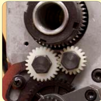
129. Check neutral gear position.
