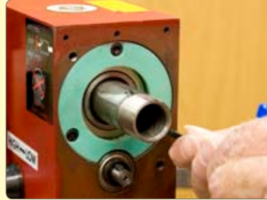
48. Remove the spindle rear bearing cover.
