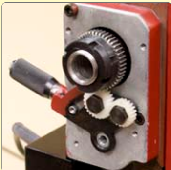
126. Fit tumbler reverse mechanism.
