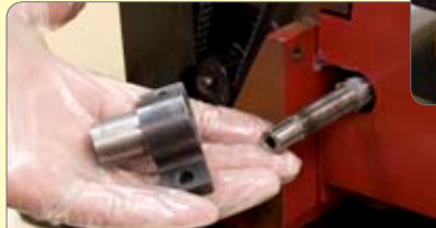
24. Remove the spacer and key from the main leadscrew.
