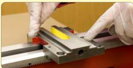
87. Drill and tap the fixing holes deeper if necessary.
