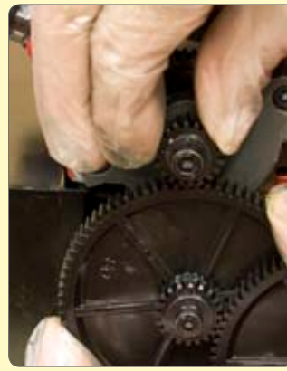
136. Engage quadrant and adjust backlash between gears A and B.
