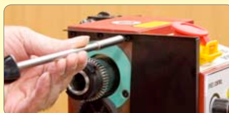
31. Remove the gear cover support bracket.
