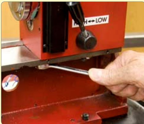
50. Undo and remove the three screws fixing the head casting to the bed and remove the head.
