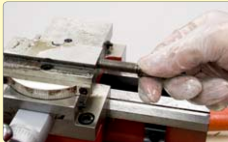
11. Unscrew the leadscrew from the compound slide base.
