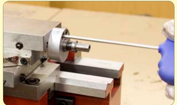
170. Adjust the screws so the slide will move back and forth easily by hand.
