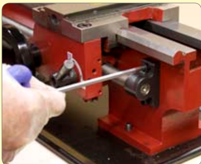
26. At the tailstock end, removed the leadscrew carrier bracket.
