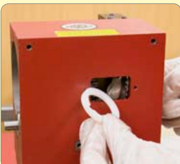
63. Make and fit a new 0.190" (4.8mm) spacer between the gear and speed encoder disk inside headstock.
