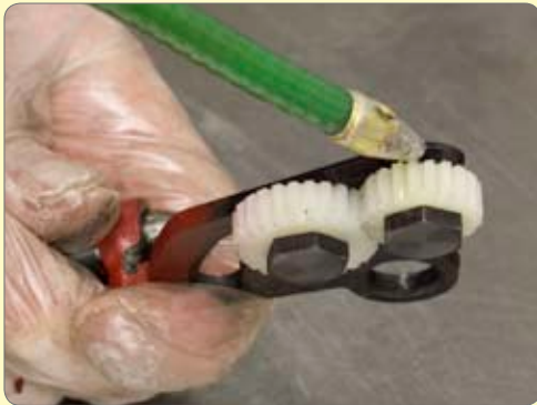
123. Oil the tumbler reverse gear shafts.
