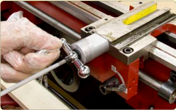
16. Remove the screw securing the cross slide handle. Remove handle and spacer.
