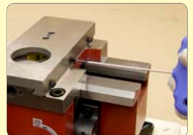
148. Fit adjusting screws lightly.
