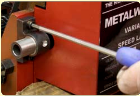
109. Loosely fit leadscrew bracket & grease bore.
