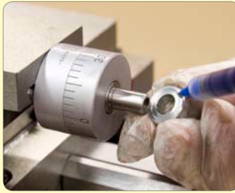
176. Backlash can often be reduced by turning a recess in the spacer to clear the shoulder on the end of the feed screw. The recess depth should be slightly less than the measurement taken with the feeler gauge to allow some clearance. Adjust for free movement with minimal backlash.
