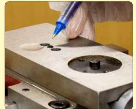
159. The centre screw is for adjusting the position of the nut in an up/down direction and the two outside screws are for locking. Slacken all three screws for now.
