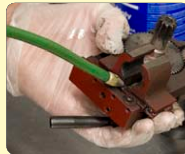
104. Oil 1/2 nut cam slots and dovetails. 105. Temporarily fit apron to saddle.
