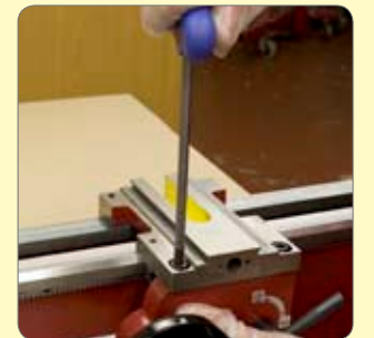
104. Oil 1/2 nut cam slots and dovetails. 105. Temporarily fit apron to saddle.
