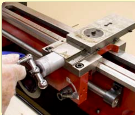
13. Wind the cross slide off the lead screw.
