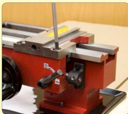
112. Slightly loosen apron fixing screws.
