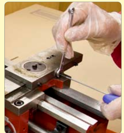
14. Slacken the gib adjusting screws.
