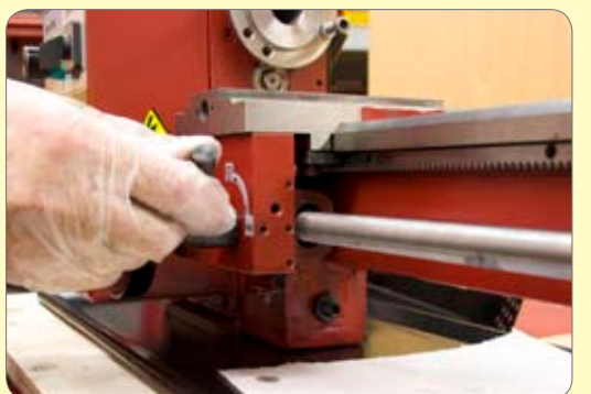
117. Move saddle to headstock end and lock 1/2 nuts.
