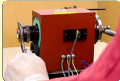
81. Adjust the bearings for "slight drag" and pinch up the C nuts for the moment. Following the Start Up Procedure on page 18, run the spindle to warm it up and settle the grease. Check and adjust the preload again. Lock the C nuts when the preload appears to be OK. Take care not to overdo the preload as this could overheat and damage the bearings.
