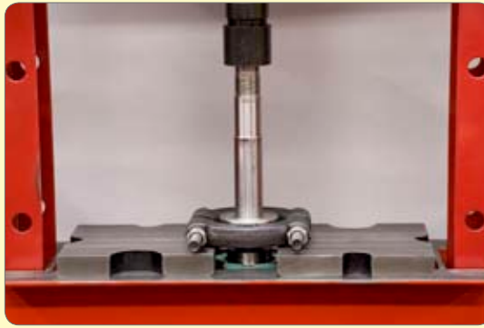
53. Press or pull off bearing and remove bearing cover from spindle. If the bearing is tight to remove, polish the spindle to make the bearing a Push Fit otherwise you will not be able to preload the taper roller bearings accurately.
