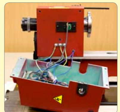
32. Remove 4 screws securing the control panel and lay to one side.
