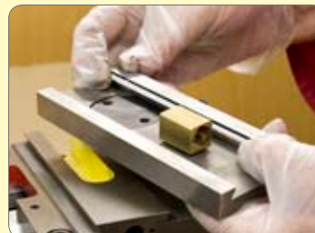
151. Drop in gib strip and lubricate all ways.
