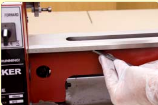
84. Scrape any paint off the bed shears.
