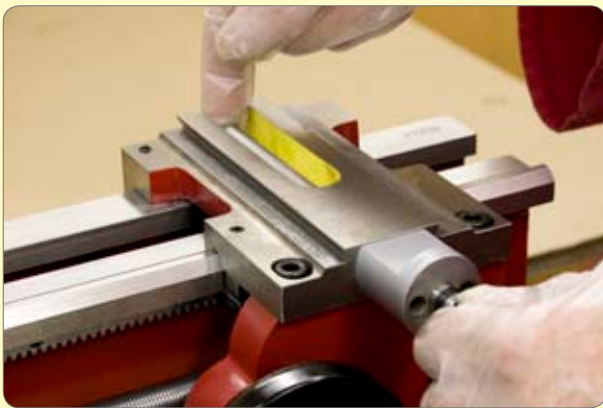
142. Temporarily fit the cross slide feed screw and bracket and check for backlash.
