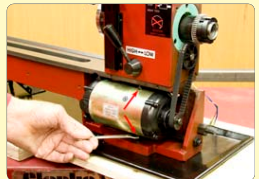
40. Slacken the two drive belt adjusting screws.
