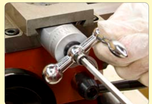
165. Refit the handle assembly.
