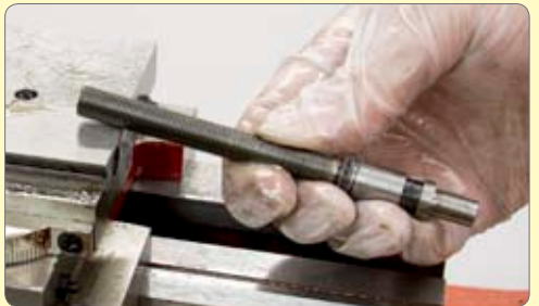
9. Slacken the gib adjusting screws.
