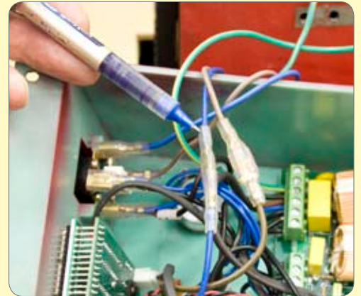
36. Disconnect the motor wires.
