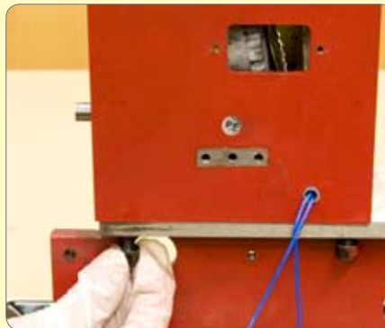
59. Refit headstock to bed making sure mating faces are clean and tighten down.
