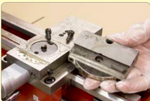
12. Remove the compound slide base.
