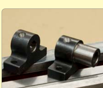
107. Drill oil holes through to the bore using a centre drill.
