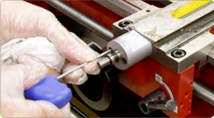
17. Remove the leadscrew end plate and leadscrew.
