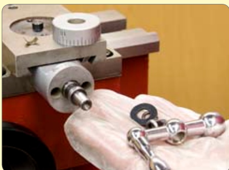
164. Remove the handle again in order to fit the micrometer dial and friction spring.
