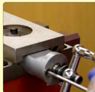
161. Pinch up the cap screws equally while winding the slide in and out until handwheel turns freely and with minimum drag. Continue adjusting all three screws until the slide moves freely along its full travel.
