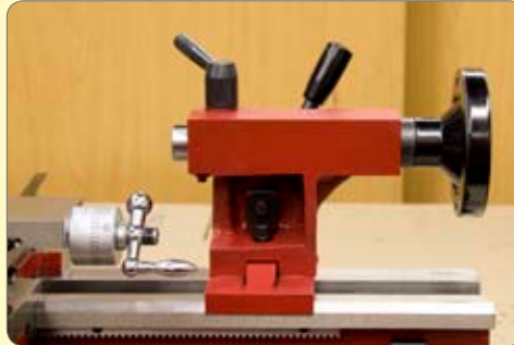
181. Fit the tailstock.
