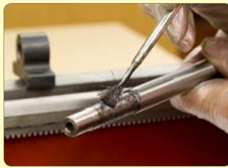
110. Grease end of leadscrew and feed through 1/2 nut and into bracket at headstock end.
