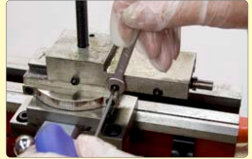
9. Slacken the gib adjusting screws.
