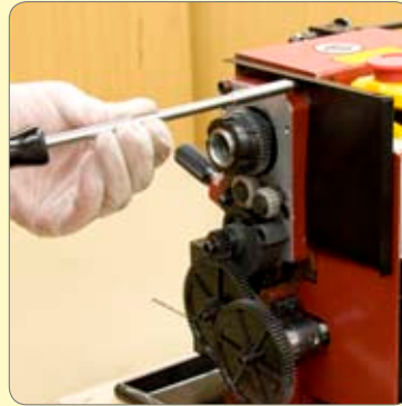
139. Refit cover support bracket.
