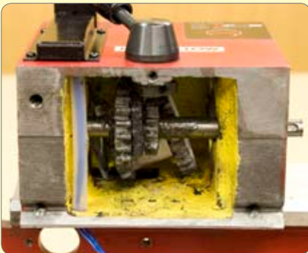
58. Apply light coating of grease to gears and gear change linkage.
