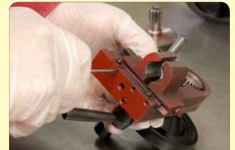
102. Adjust the gib screws if necessary.
