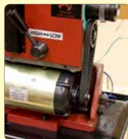
75. Refit the drive belt and adjust tension. If you cannot twist the belt through 90° quite easily, the tension is probably too tight.
