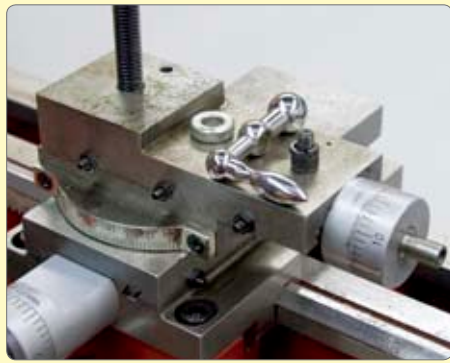
6. Remove the screw securing the compound slide handle. Remove handle and spacer.
