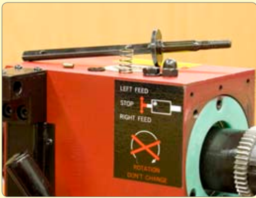
43. Remove the chuck guard carrier spindle etc.
