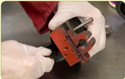
100. Check 1/2 nuts are correctly adjusted on apron by operating lever.
