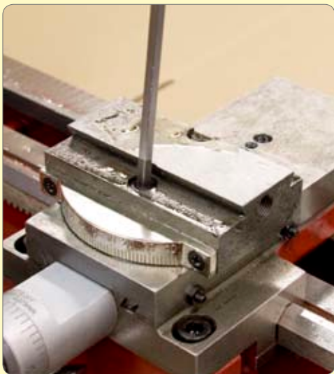
10. Remove compound slide and gib strip.
