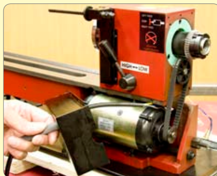
37. Disconnect the mains supply leads from the em-stop switch.
