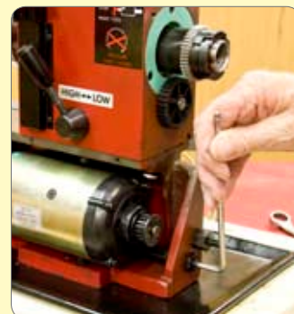
42. Undo the motor mount pivot screws enough to remove the motor.
