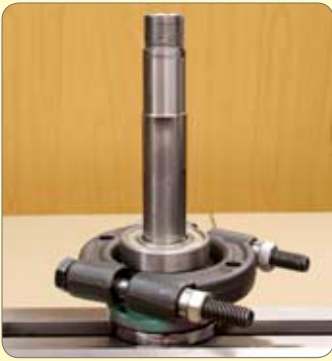
53. Press or pull off bearing and remove bearing cover from spindle. If the bearing is tight to remove, polish the spindle to make the bearing a Push Fit otherwise you will not be able to preload the taper roller bearings accurately.
