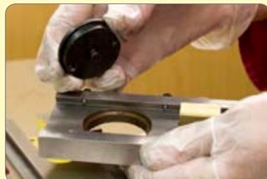
150. Fit top slide base retaining plate.
