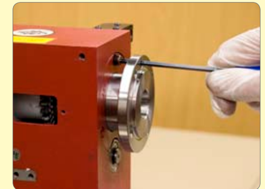
73. Secure front bearing cover.
