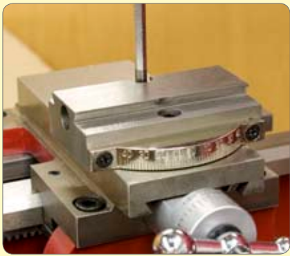
166. Fit compound base to cross slide.
