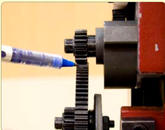
132. Check for correct gear alignment.
