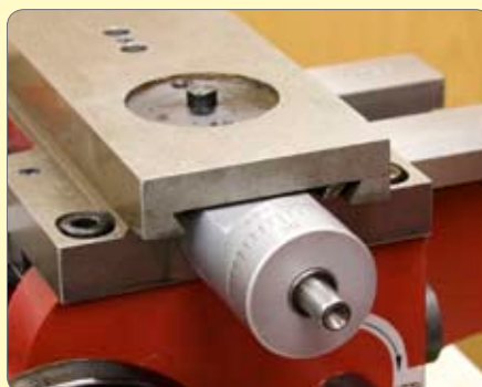
164. Remove the handle again in order to fit the micrometer dial and friction spring.
