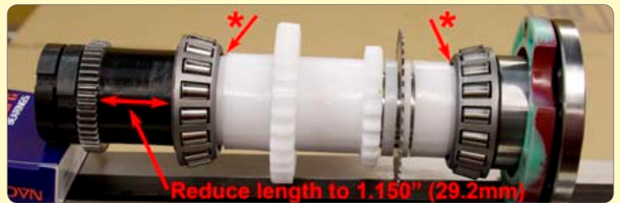
62. This picture shows the complete sequence of parts loosely assembled on the spindle. Gaps are left to clearly show the parts. There will be no gaps when assembled in the head. * Note the outer spacers require a shoulder turning to clear the bearing cage.
