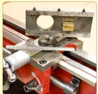
14. Slacken the gib adjusting screws.
