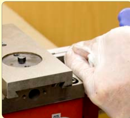
153. Fit adjusting screws and adjust so slide can be moved back and forth easily by hand.
