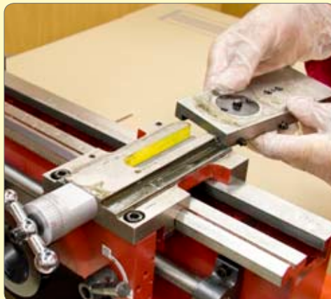
15. Pull off the cross slide assembly.
