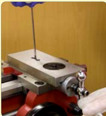
158. Wind the cross slide in and out. If there is any tightness, the feed screw nut will need adjusting.
