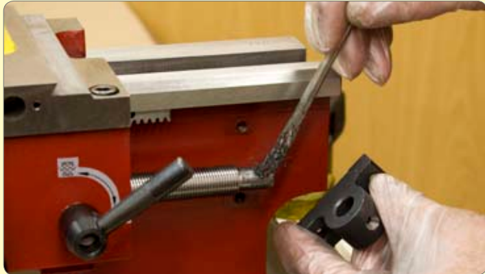
111. Grease end of leadscrew and bracket bore and temporarily fix in place.
