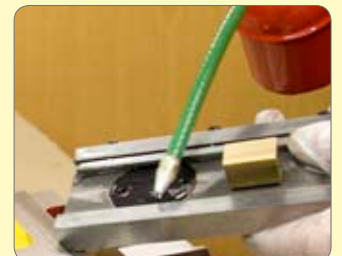
148. Fit adjusting screws lightly.
