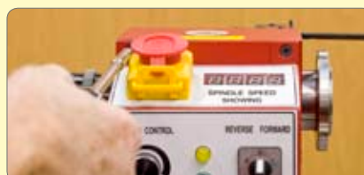
32. Remove 4 screws securing the control panel and lay to one side.
