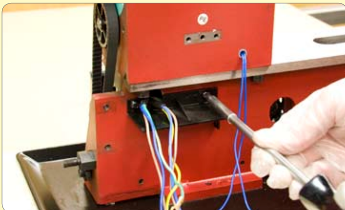
77. Refit the cable protector.
