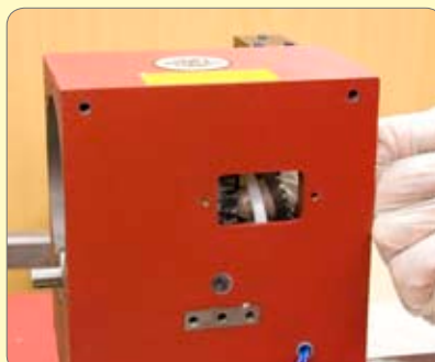
63. Make and fit a new 0.190" (4.8mm) spacer between the gear and speed encoder disk inside headstock.
