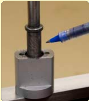
154. Grease / oil the feed screw and bracket.
