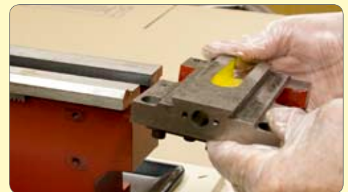
29. Slacken the saddle adjusting screws and slide the saddle off the end of the bed.
