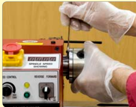
4. Remove the chuck.
