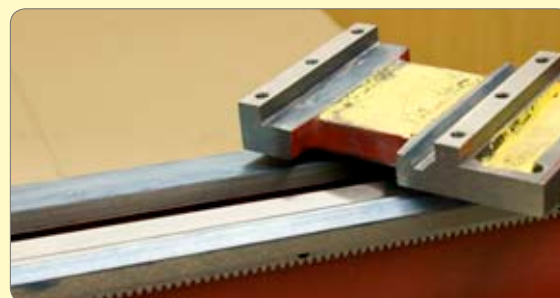
89. Place the saddle on the bed and check to see how it sits.
