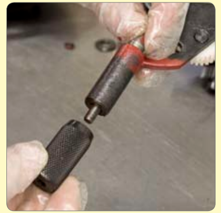
122. Strip, clean, oil / grease and reassemble the tumbler reverse detent assembly.
