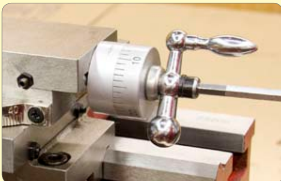
174. Fit the spacer and handle and wind the slide back and forth.
