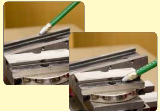
168. Oil top slide assembly and fit.
