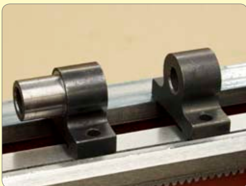
106. The leadscrew brackets as they come on the machine. Notice there is no means of lubricating the bearing surfaces other than at each end of the bracket.
