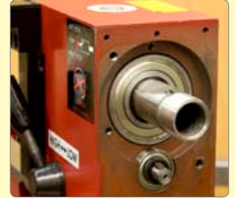
45. Using two C spanners, unlock & remove spindle nuts.
