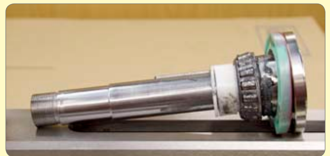
64. Refit the key, the original spacer + the small 0.110" (2.8mm) thick spacer (the original small spacer reduced in thickness) to the spindle and grease the bearing.
