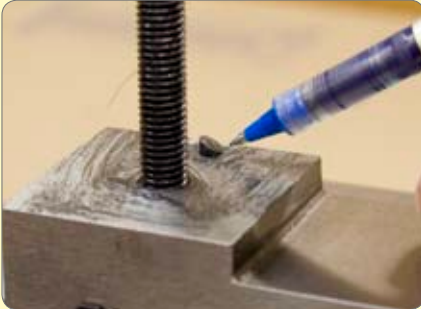
178. Grease and fit the tool post spring and plunger and fit the tool post.
