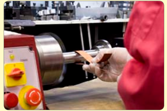
54. Polish the spindle and test the fit by using one of the old bearings (if not damaged).
