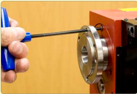
49. Using a hole in the spindle flange for access to the 3 fixing screws, remove the front bearing cover.
