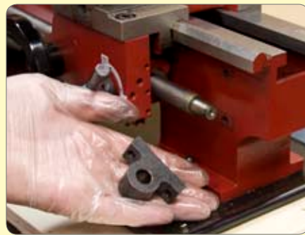
26. At the tailstock end, removed the leadscrew carrier bracket.
