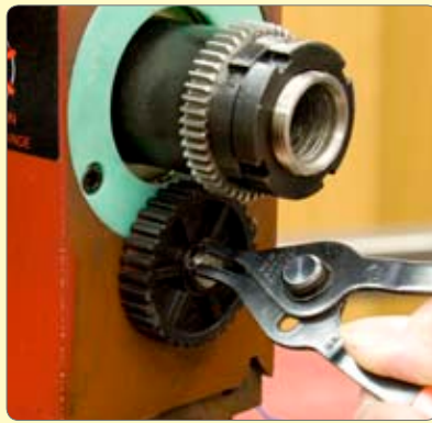
44. Remove circlip & pull off drive pulley.
