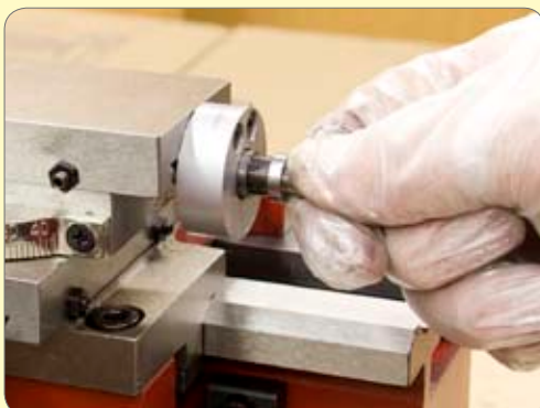
172. Turn the feed screw to check it turns freely.
