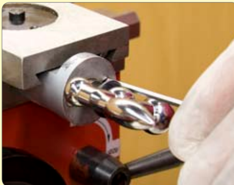
157. Slacken the bracket screws, wind the slide right back and tighten the screws.
