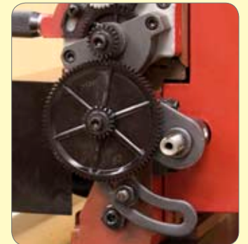
131. Refit lower gear quadrant.
