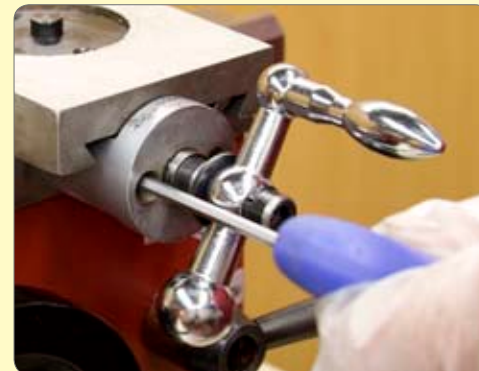
157. Slacken the bracket screws, wind the slide right back and tighten the screws.
