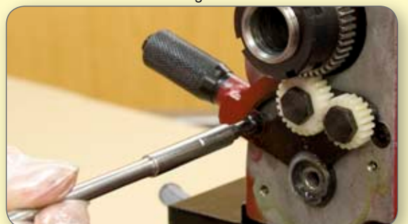
22. Undo and remove the tumbler reverse arm.
