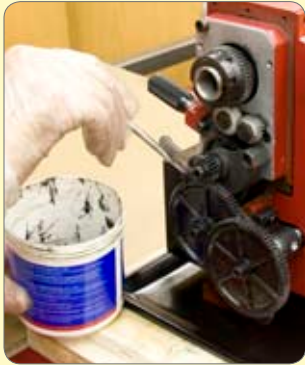
137. Very lightly grease gears.
