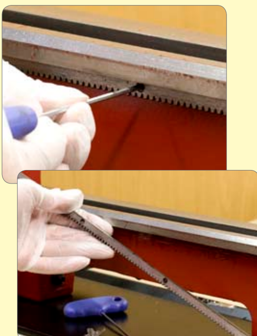
30. Remove the rack from the front of the bed.
