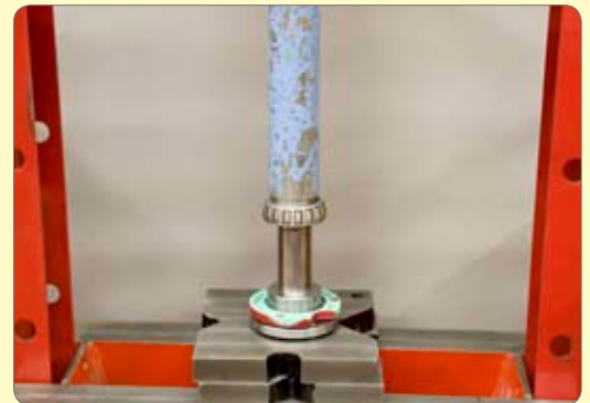
60. Refit front bearing cover to spindle and press on new 30206 taper roller bearing inner
