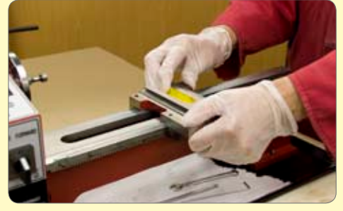
99. Test slide saddle up and down the bed. There should be slight drag with no free play. Lightly pinch up remaining cap screws checking after each one and adjusting as required.
