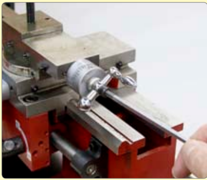
6. Remove the screw securing the compound slide handle. Remove handle and spacer.
