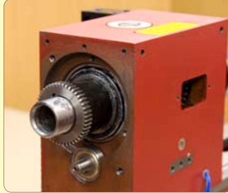
69. Fit metal drive gear.
