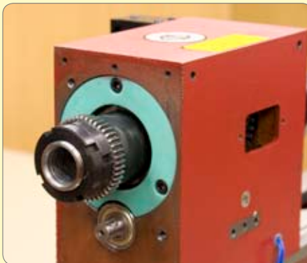
71. Fit rear plastic bearing cover.
