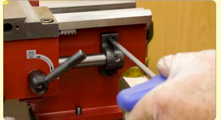
110. Grease end of leadscrew and feed through 1/2 nut and into bracket at headstock end.
