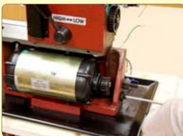
74. Refit the motor onto it's pivot screws.
