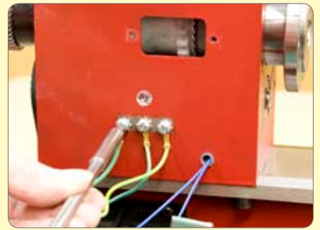
34. Disconnect the three earth wires.
