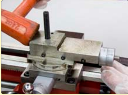
7. Tap compound slide along with a soft mallet to remove micrometer dial and friction clip.
