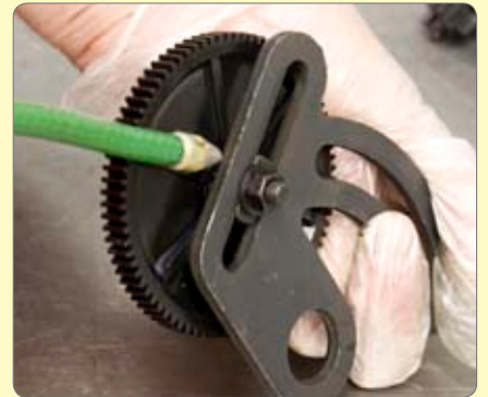
125. Oil the lower quadrant gear shaft.
