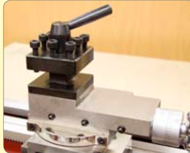
178. Grease and fit the tool post spring and plunger and fit the tool post.
