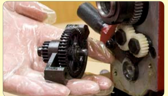
...and remove the transfer gear carrier.
