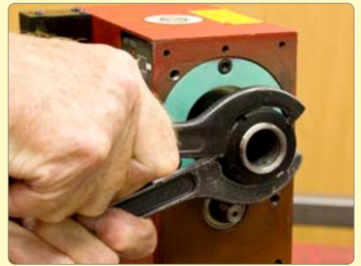
45. Using two C spanners, unlock & remove spindle nuts.
