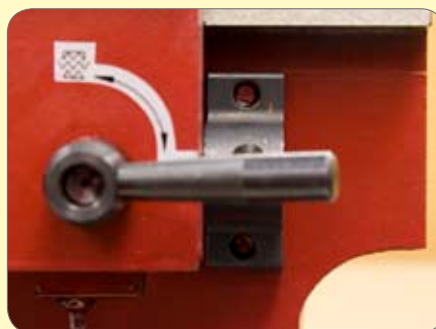
116. Check the bracket holes align with the holes in bed. If holes are misaligned, slot the bracket holes to correct and refix screws.
