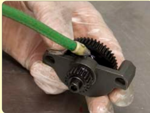
124. Oil gear shaft.
